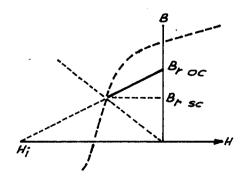
Fig. 1. Demagnetization graph for a permanent magnet.
