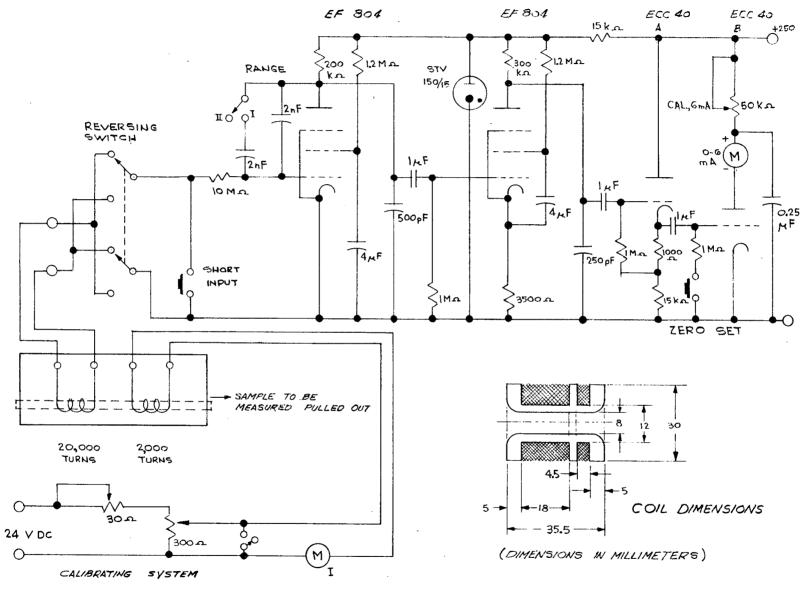
Fig. 5. Schematic diagram of electronic fluxmeter, circuit for calibrating it, and construction of induction coil.
