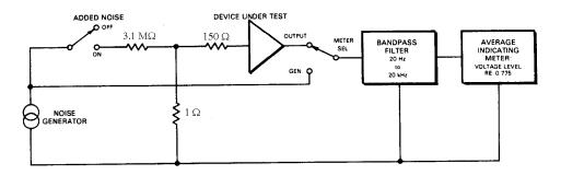
Figure 2: Practical setup for a direct-indicating measurement of the noise index by the "noise generator method." These particular values hold only for a source resistance of 150 cc, bandwidth of 20 kHz, and an average-indicating meter of voltage level re 0.775 V. (A balanced circuit could be used if needed.)
